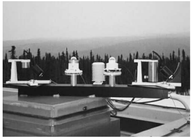
Figure 1. Multi-Filter Rotating Shadowband Radiometers (MFRSR) and broadband radiometers at the long-term monitoring site on the roof of the Davis Science Center of the Geophysical Institute, University of Alaska, Poker Flat Research Range.
